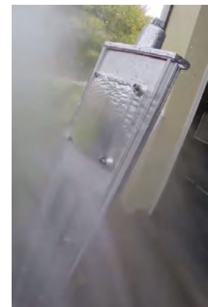
Our Pauluhn DLL LED linear undergoing 2000psi high pressure hose test at 5 feet (1.5m) for 30 minutes
