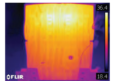
Thermal images of Champ-Pak CPMV LED wall pack
